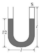
All of mercury can be displaced from the tube by heating slowly the gas in the sealed end of the tube, which is separated from the atmospheric air by mercury. Determine the work done (in joule) by the gas there by if the atmospheric pressure is  $P_0 = 10^5$  Pa, the density of mercury is  $\rho_{\text{mer}} = 13.6 \times 10^3$  kg/m<sup>3</sup>, and the cross-sectional area of the tube is S = 1 cm<sup>2</sup>.
